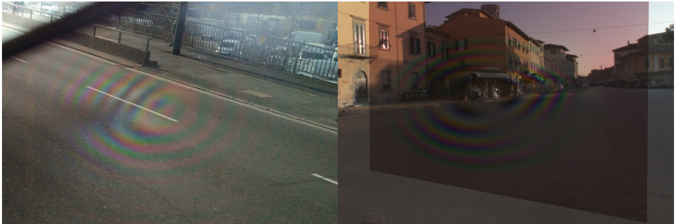
Figure 1: (Left) Photo captured through the window of a train using a common handheld device and viewed through the polarising lens of a pair of sunglasses. The window exhibits stress-induced birefringence which gives rise to the visible iridescence. Notice that the visual effect is most powerful when the incident light is reflected off the road as light reflected around the Brewster's angle is strongly polarized. (Right) An optically anisotropic slab rendered using our method and exhibiting iridescence induced by birefringence as well. Incident light was assumed to be partially polarized.
